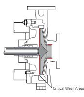
Area Nose Ring =  $2\pi rW$  = 2  $x\pi x(.9)$  (.9) = 5 in<sup>2</sup> Area Back Cover =  $\pi r^2 = \pi (5)^2 = 79$  in<sup>2</sup> Total Wear Area = 5 + 79 = 84 in<sup>2</sup>
