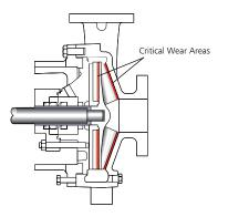
Wear Area Calculation (10 inch dia. impeller) Area Wear Surface =  $\pi r^2 = \pi (5)^2 = 79 \text{ in}^2$ Total Wear Area (Front & Back) =  $2x 79 = 158 \text{ in}^2$
