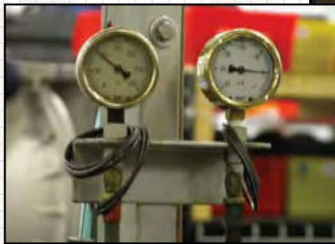
Experienced Warren Rupp assembler monitors pump performance with pressure and vacuum gauges.
