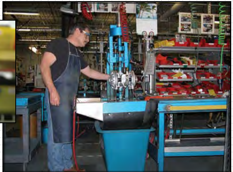
Experienced Warren Rupp assembler monitors pump performance with pressure and vacuum gauges.
