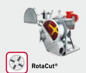
Macerator and heavy material separator in one. Reliably separates foreign matter such as stones or metal parts and effectively macerates fibrous and course matter in liquid media, thereby ensuring more homogeneous and flowable suspensions.
