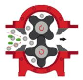
Injection S: Symmetrical pump housing segments with the InjectionSystem design, arranged on the discharge and suction sides
