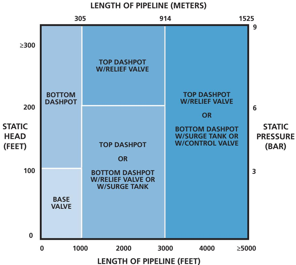
The application graph illustrates the range of use for three valve configurations: 1) base valve, 2) bottom mounted oil dashpot, and 3) top mounted oil dashpot. For example, on a 2,500 ft. long water transmission main operating at 150 ft. of head, a Tilted Disc Check Valve with a top mounted oil dashpot would be selected. Or, if a surge relief system is provided, then the bottom mounted oil dashpot configuration may be used.
