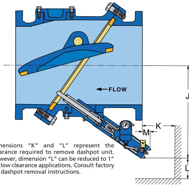
Dimensions "K" and "L" represent the clearance required to remove dashpot unit. However, dimension "L" can be reduced to 1" for low clearance applications. Consult factory for dashpot removal instructions.
