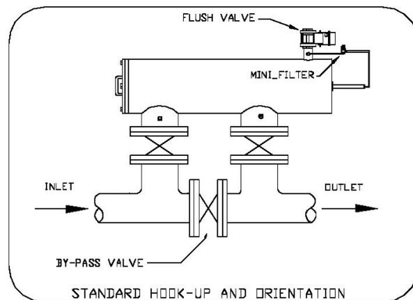
Flush line pipe must be ridged. It should not be made out of flexible tube or rubber hosing. Any restrictions in the flush line will reduce the cleaning ability of the filter.
