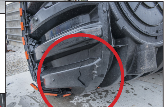
Tank cracked, clips on seam were dislodged.
