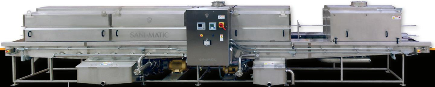
**The Sani-Matic Tunnel Wash** is an automated tunnel washer designed to clean a wide variety of high-volume items such as pans, totes, pails, buckets and trays. The basic design includes detergent and final rinse zones. Pre-rinse and recirculated rinse zones may be provided for heavy product residues or high-capacity requirements.
