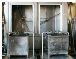
Left: The compact single-position buggy washer allows closer location to production
