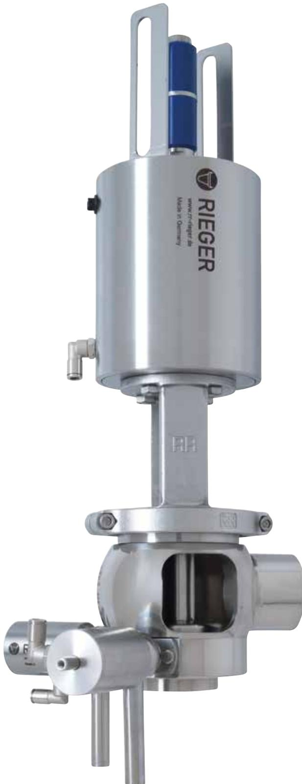
Rieger double seal valves are used for reliable separation of product from cleaning agent. The leakage space is situated between the separating gaskets. The leakage fluid flows through two leakage valves.
