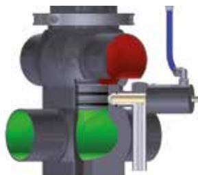
Two-way connection between main and CIP valve
