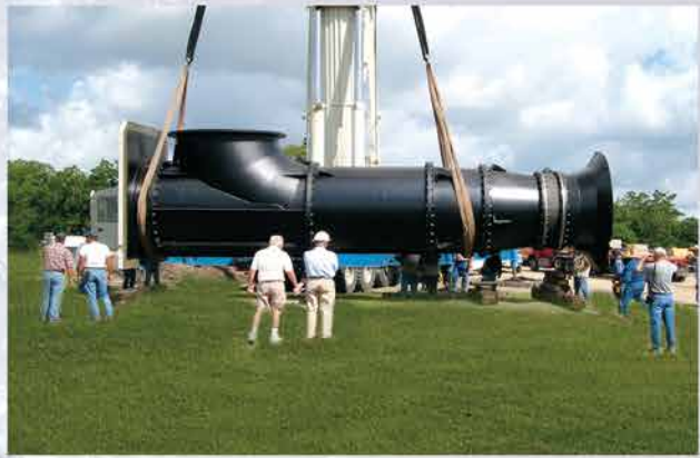
Available in open or enclosed line shaft configurations. Enclosing tubes, when used, are schedule 80 and are supported by spiders when required by the pump length.
