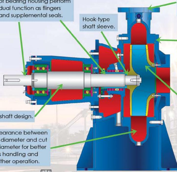
V-Ring flingers at each end of bearing housing perform dual function as flingers and supplemental seals.
