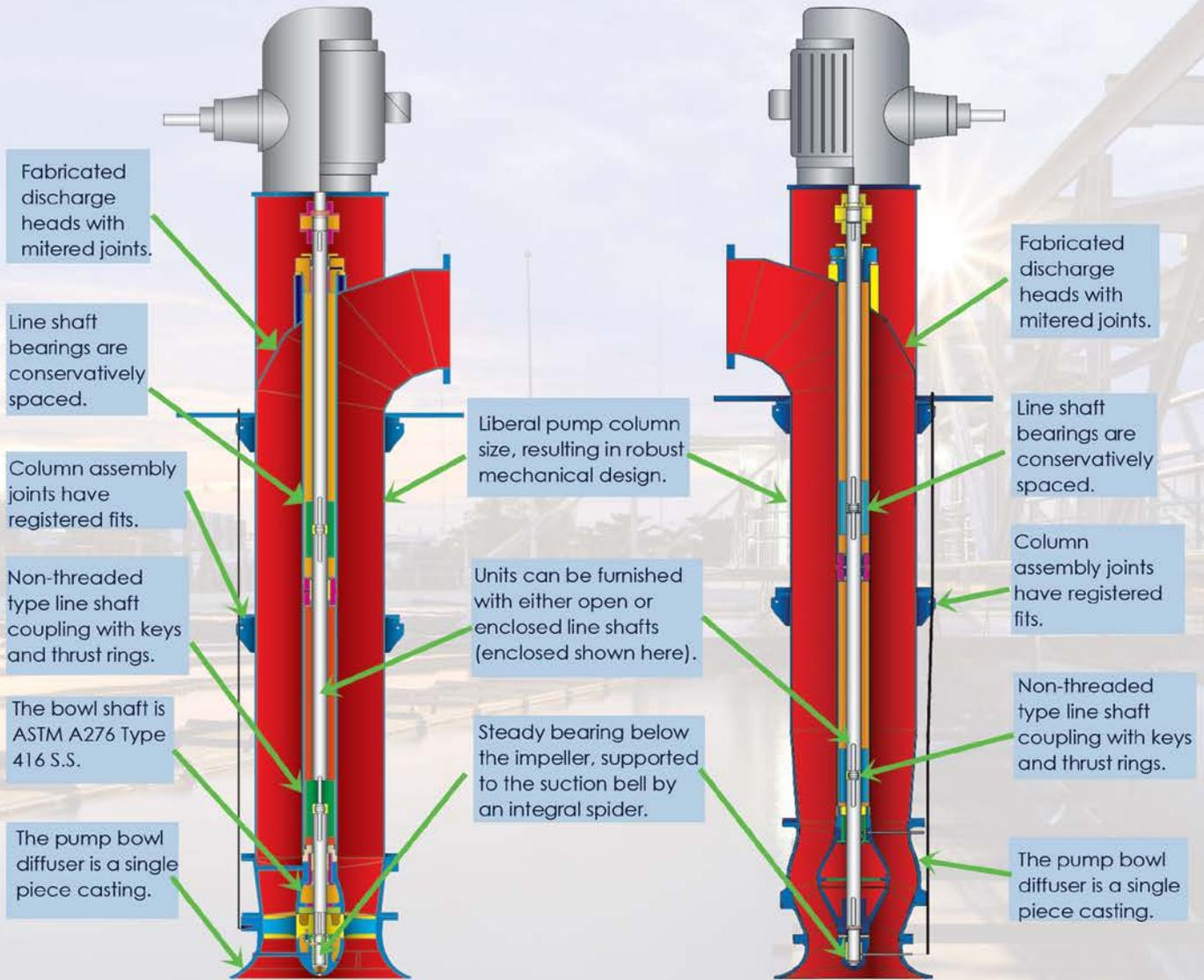
Available in open or enclosed line shaft configurations. Enclosing tubes, when used, are schedule 80 and are supported by spiders when required by the pump length.
