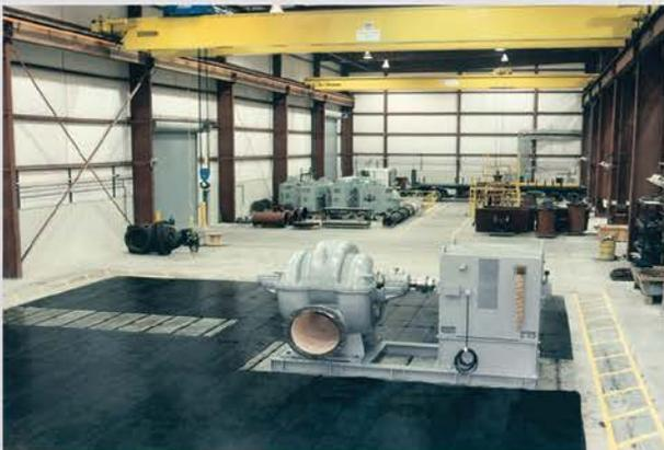
The test facility is not only large, but it also features a comprehensive range of testing equipment to ensure both mechanical and hydraulic performance. With this enormous capacity, pumps can be tested for a wide variety of simulated field conditions. Then, from the assembled test data, it is an easy matter for computers to generate values of pump capacity, head, horsepower and efficiency.
