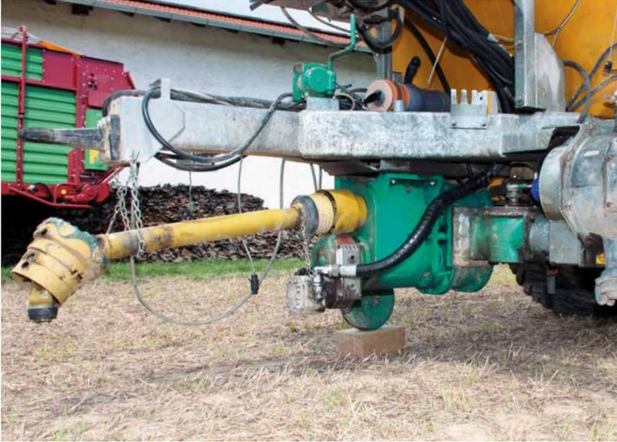
Spraying liquid manure at a flow rate of 5000 l/min, the pump being driven from a tractor via a PTO shaft. Other capacities available.
