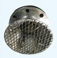
Breaks swirl and helps present a laminar flow to the suction inlet which reduces chance of cavitation.
