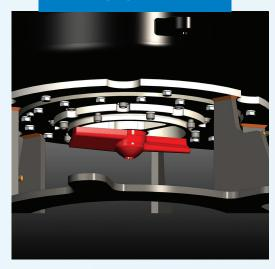
This wholly independent chopper unit features heavy duty blades, located in front of the pump's suction. Best of all, because the chopper unit is independent of the impeller, as the unit dulls or wears, it can be replaced without having to replace the whole impeller assembly.
