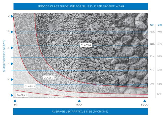
The above chart is for use as a guide only. It assumes 2.65 Ss silica-based solids. Adjust rating to account for solids of different abrasivity using ASTM G75-95. The chart is based on the Hydraulic Institute's Slurry Class guideline. For more information about the HI Slurry Classes please visit http://pumps.org or call HEVVY PUMPS for assistance.
