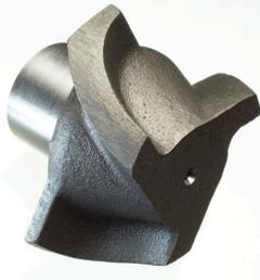
Heavy duty blades, situated in front of the pump's suction, agitates, chops, cuts, shreds incoming solids such as metal banding, plastic, wood, rags and bags, prior to them entering the impeller. The 'chopper' eliminates pump and system downtime by preventing the plugging of pump suctions and pipelines.
