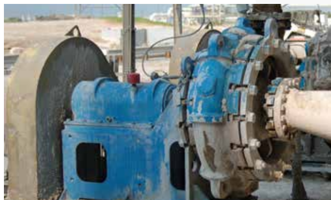
Model 5500 pumping Phosphogypsum in a phosphate plant.
