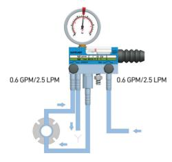
Changes in the pre-set system values for flow and pressure will indicate any possible problems in seals and system well in advance. For automatic control, alarm sensors can be used.
