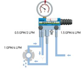
Safeunit system also detects seal water leakage in the process resulting in extra heating and evaporation costs or expensive quality problems such as dilution.
