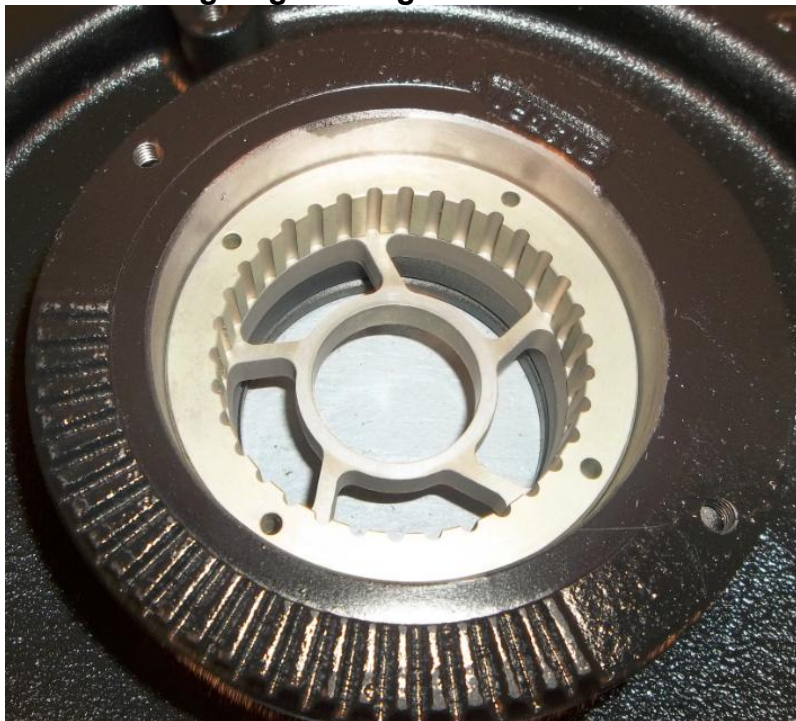
Radial shredder ring installed.
