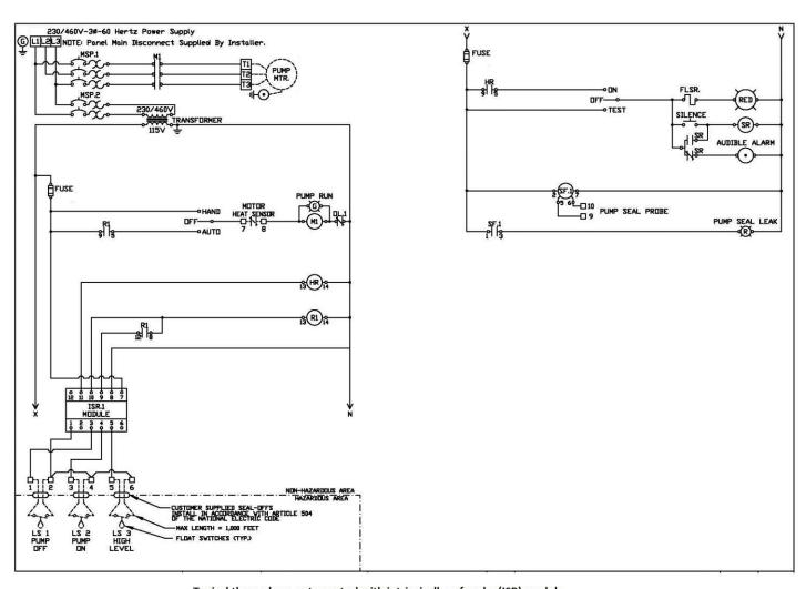
Typical three phase auto control with intrinsically safe relay(ISR) module and with seal minder & thermal sensor connection.
