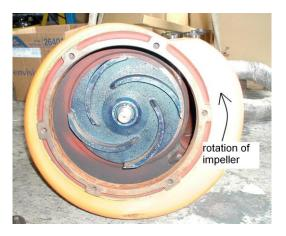
2. By looking from the top of the pump. Since the impeller cannot be seen, the best way to check the rotation is to check the kick back motion of the pump when the pump just starts. The kick back motion of the pump should be counter clockwise as shown in the picture below.
