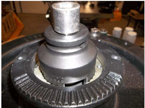
The shredder cutting bar should be tightened to the proper torque using the special socket tool on an impact driver.
