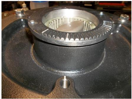
Rotate the shredder housing clockwise 6 markers.
