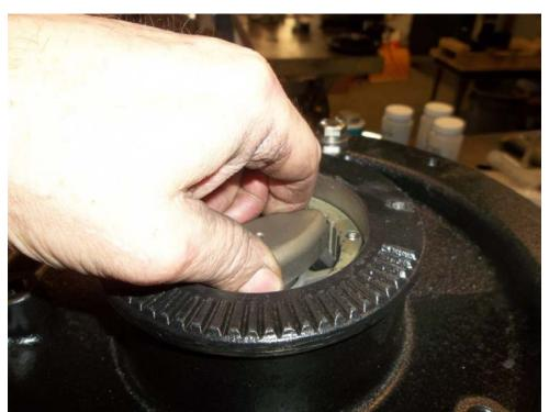
Once the shredder cutting bar has been tightened to the shaft, verify that it can spin freely. The cutter elements are sharp, so care should be taken not to cut fingers.
