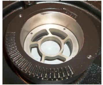
Axial shredding ring with leg slanted counter clockwise.
