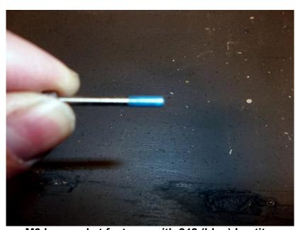
M3 hex socket fastener with 242 (blue) Loctite.
