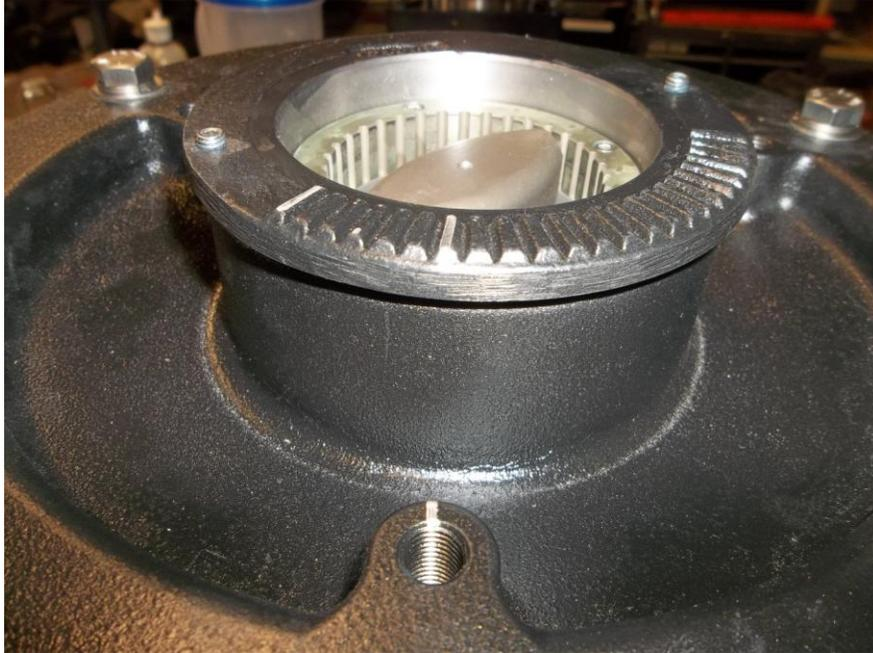
**Rotate the shredder housing clockwise 6 markers.**
