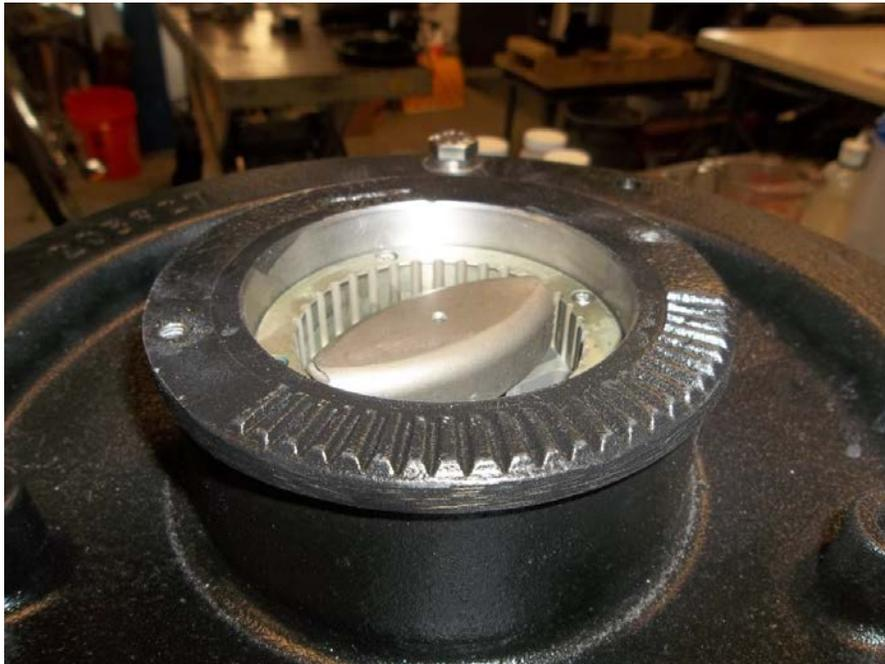
**With the housing threaded completing into the suction cover, the shredder cutter bar can be threaded onto the shaft to retain the impeller.**
