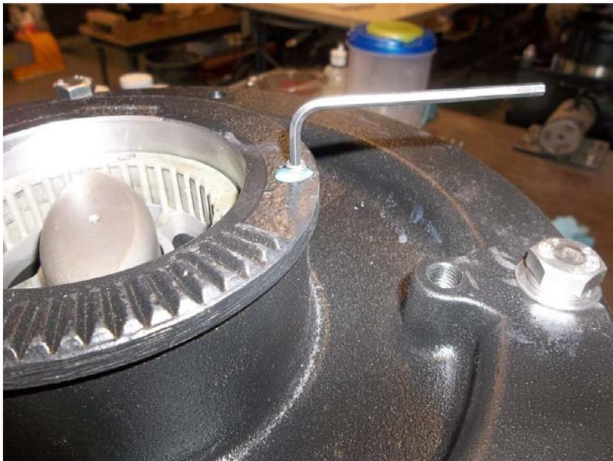
**Thread the locking screws down until contact is made with the suction cover.
