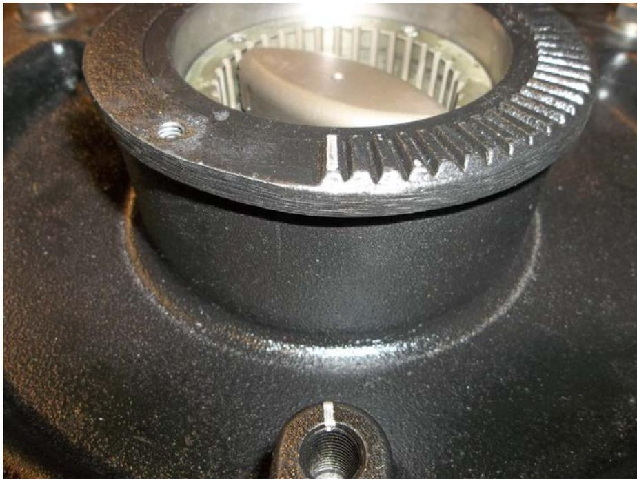
**Mark the point where the stationary axial shredding ring interfaces with the shredding cutter bar.**
