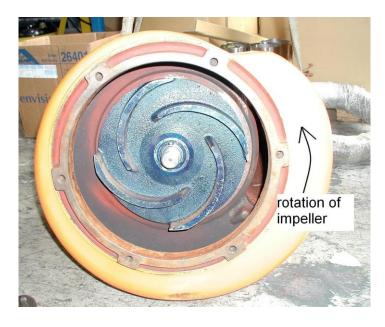
2. By looking from the top of the pump. Since the impeller cannot be seen, the best way to check the rotation is to check the kick back motion of the pump when the pump just starts. The kick back motion of the pump should be counter clockwise as shown in the picture below.
