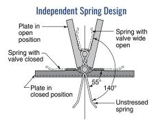
A spring design of the DUO-CHEK® (sizes 6" and larger) allows higher torque to be exerted against each plate with independent closing in response to the process stream. Testing has proved this action provides up to 25% improvement in valve life and 50% reduction in water hammer.
