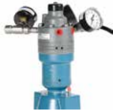
Pneumatic Moore Positioner with Gauges
